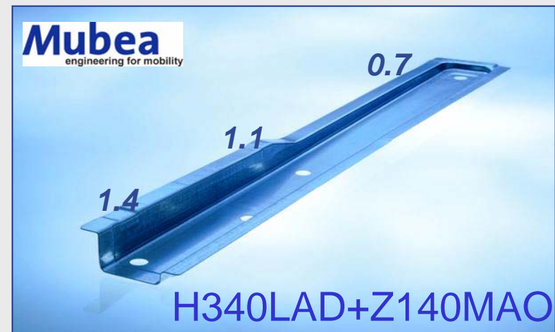
Tailored rolled: 1.4 to 1.1 mm to 0.7 mm
